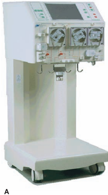
Figure 44-6 Devices for administering continuous renal replacement therapy (CRRT) offer an integrated fluid warmer for the heating of infusion and dialysate fluids, a weighing system to reduce the possibility of error in assessing fluid balance, and a battery backup that allows treatments to continue when the patient is moved. A , Diapact CRRT System, B-Braun Medical, Inc., Bethlehem, PA. B , PRISMA, Gambro Corporation, Lakewood, CO.
